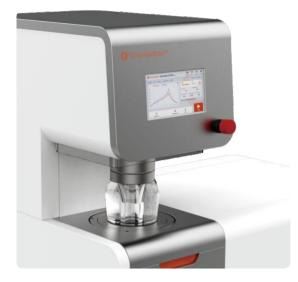
One pre-test can accurately control the bursting speed The full servo hydraulic system is controlled by Al algorithm, together with precise screw drive, only by one pre-test, the machine can reach the expansion speed within the standard requirements of 20s.
