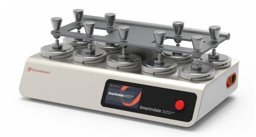
The Smartindale is used for abrasion and pilling tests on You can switch the abrasion and pilling tests with a one-
