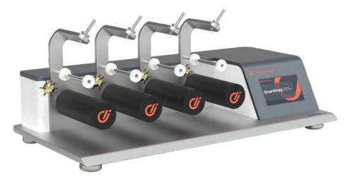
SmartSnag checks how easily a fabric can be hooked under normal wear. For evaluating the degree of hooking of outerwear and other fabrics, especially those made of chemical fibers or filaments.
