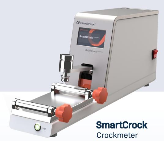
SmartCrock Crockmeter is used to test the color fastness of textiles or leather to dry or wet rubbing. In the test, a standard white rubbing cloth is rubbed repeatedly against a sample at a certain speed. After the test, you can rate color fastness by comparing the color depth of the friction cloth with the standard grey card. They do this under a standard light.
